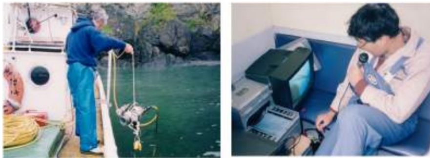
Fig. 9. Photos showing video camera system for sea-truthing in Akkeshi Bay, east Hokkaido. Underwater video camera is lowered from the boat (left photo). An observer monitors bottom features by the display in the cabin (right photo).
